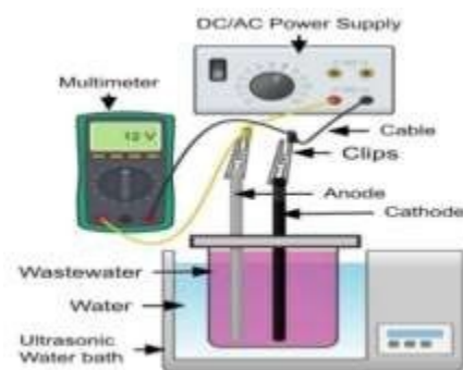
Figure 1. Hybrid sono-electrocoagulation technology (Asaithambi et al., 2024)
