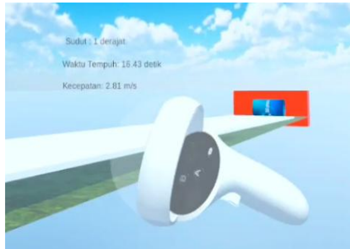
Figure 5. Results Display Panel showing Travel Time (s) and Final Velocity (m/s); values are example outputs from scenario angle=1°.
