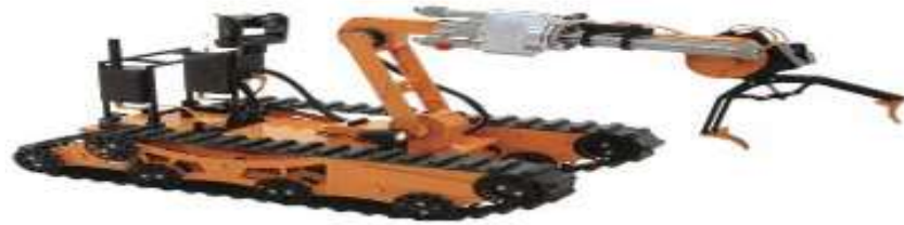
Robot Vanguard™ MK1 (Penjinak bom) (Sumber : S.costo,2004. A new robotic unit for onboard airplanes bomb disposal)
