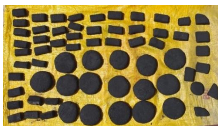
Figure 4. Printing and drying walnut shell briquettes
