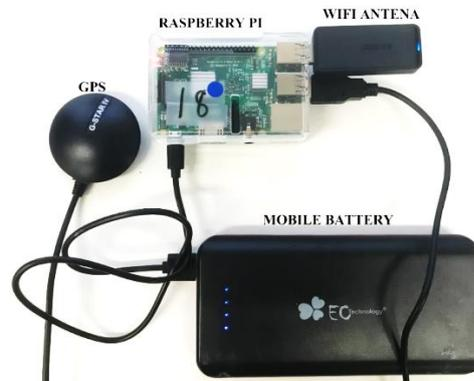
**Figure 3.** WiFi Scanner, GPS and Mobile Battery
