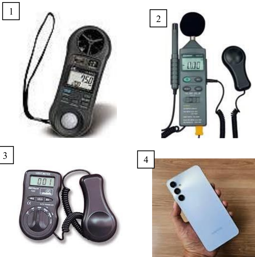
Gambar 5. (1) Digital anemometer merk Lutron LM-8000, (2) Multi-function Environment Meter merk Krisbow KW06-291, (3) Lux Meter, (4) HP
